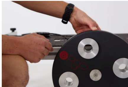
Press inward until the mass is in line with the flywheel
