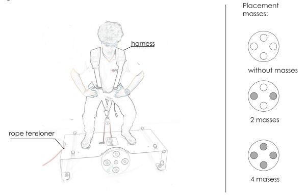
Before you start standing on the machine fully stretched, we must tighten the rope.
