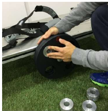
Press inward until the mass is in line with the flywheel
