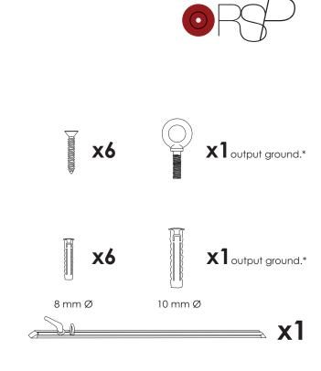
$\ensuremath{^{*}}$  This ringbolt mounting (optional) is used to derive the output block to the ground.
