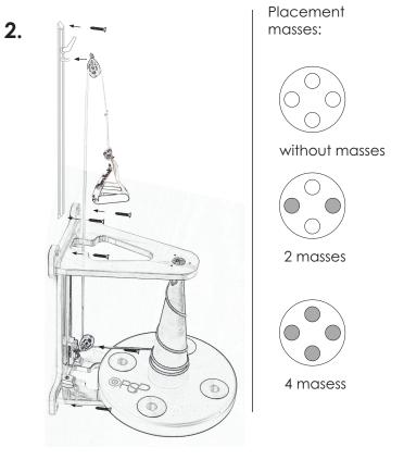
Make four holes in the wall to the height indicated, first insert the plugs and screw the four screws into the wall. Then install the rail to the block of wall outlet to the height indicated, with the plugs and screws indicated.
