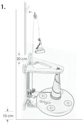
Place de machine as close as possible to the ground, if you have baseboards will be placed above it. The rail of 120 cm is placed centered with the machine and 20 cm of it.
