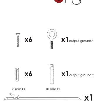
\* This ringbolt mounting (optional) is used to derive the output block to the ground.
